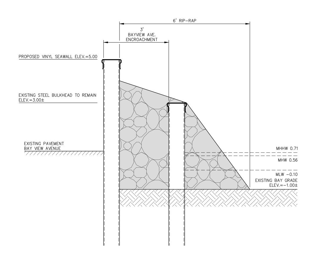
PROPOSED SEAWALL AT EXISTING BULKHEAD SECTION C-C SCALE: 3/4"=1'-0"
